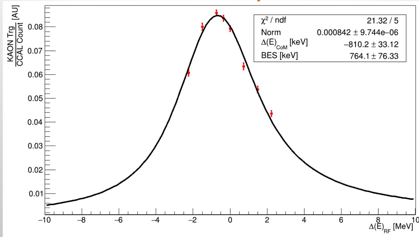
Energy scan as a function of the absolute energy deviation w.r.t. the starting point of the scan, the fitting function includes radiative corrections and the beam energy spread is left as free parameter.
