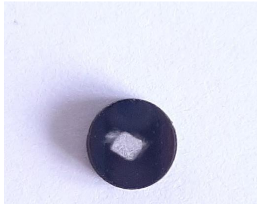
Cathode based on the IrCe alloy
