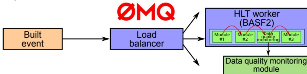
DAQ systems have a lot of components. The stability of these components has to be continuously monitored.
