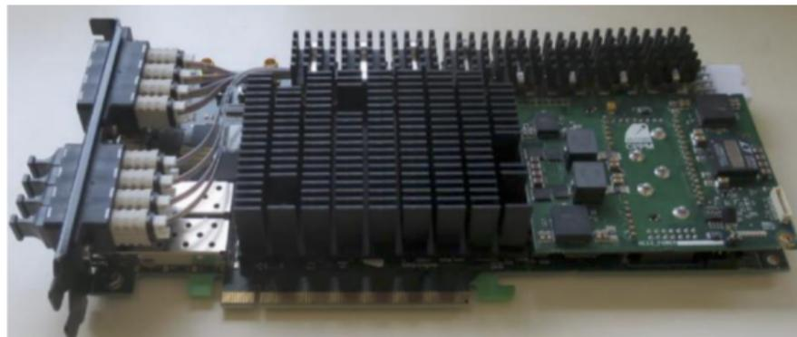
PCI-express based high-speed readout for the Belle II DAQ upgrade
