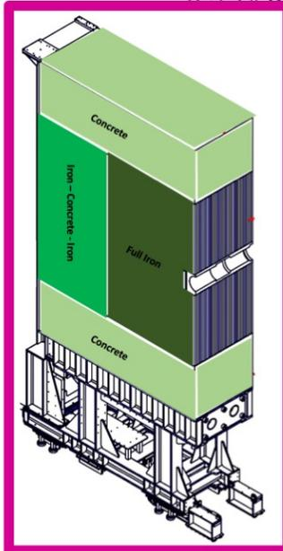
REPLACE HCAL by Iron-concrete shielding
