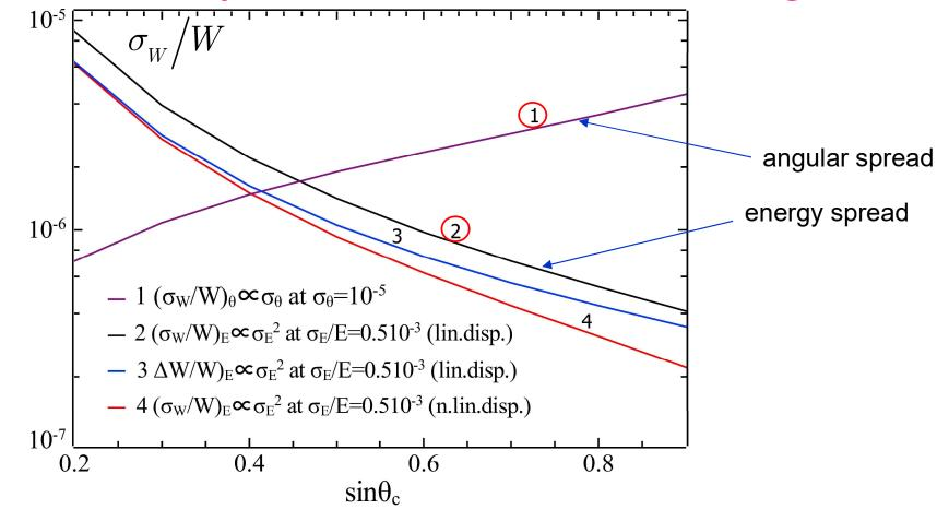
The optimum choice of the crossing angle depends on the achievable horizontal angular spread.
