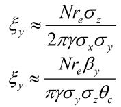
As result, attainable  $L_{c-w} \ge 20L_h$  is possible. To obtain this gain the beams should have very small transverse emittances, especially the vertical one.
