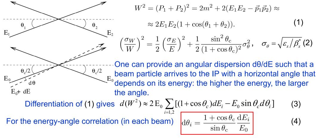
the beam energy spread does not contribute to the W spread,  $d(W^2)=0!$
