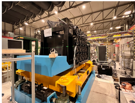
Figure 2: The AHCAL prototype installed at the SPS beamline.
