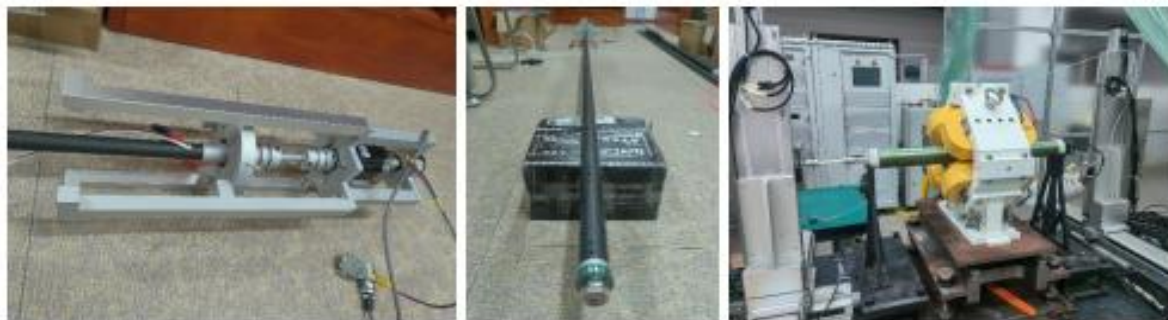
The finished rotating probe and calibrated in PM magnet, by SSRF
