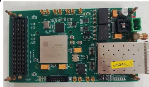
FPGA data source board
