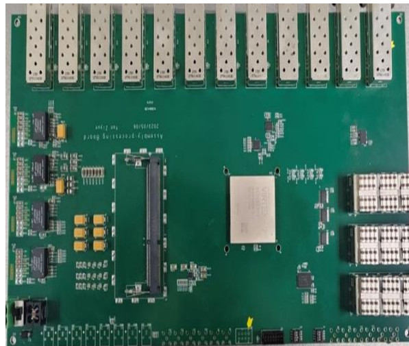
Data aggregation and processing board Prototype for Vertex detector
