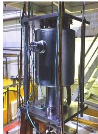
166.6 MHz超导高频原型腔
