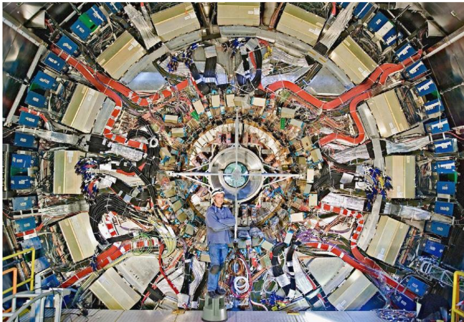
ATLAS barrel detector (Power cable: Red)
