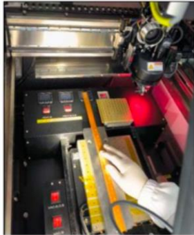
Ladder on wire bonding machine
