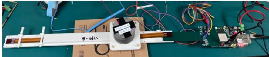
The first vertex detector (prototype) ever built in China
