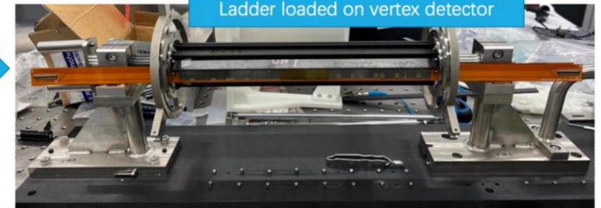
Ladder loaded on vertex detector
