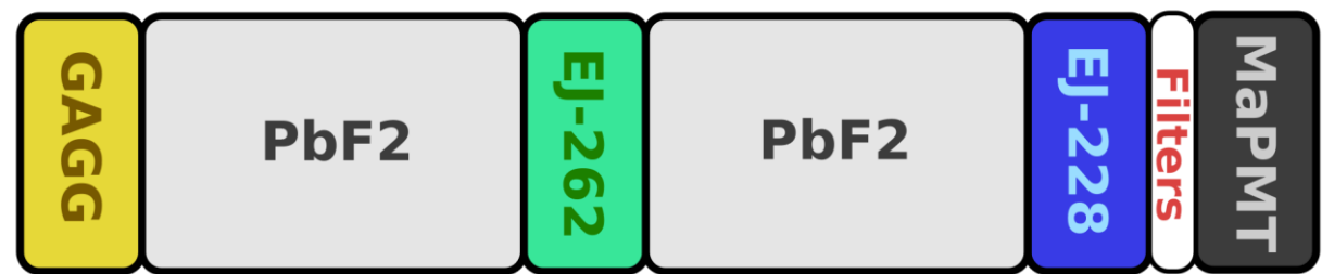
Option 2: Hybrid approach (heterostructure*) polymer layers doped with QDs interleaved with crystals.
