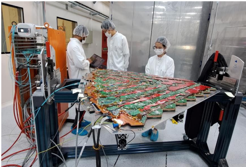
Cassette testing during assembly at CERN
