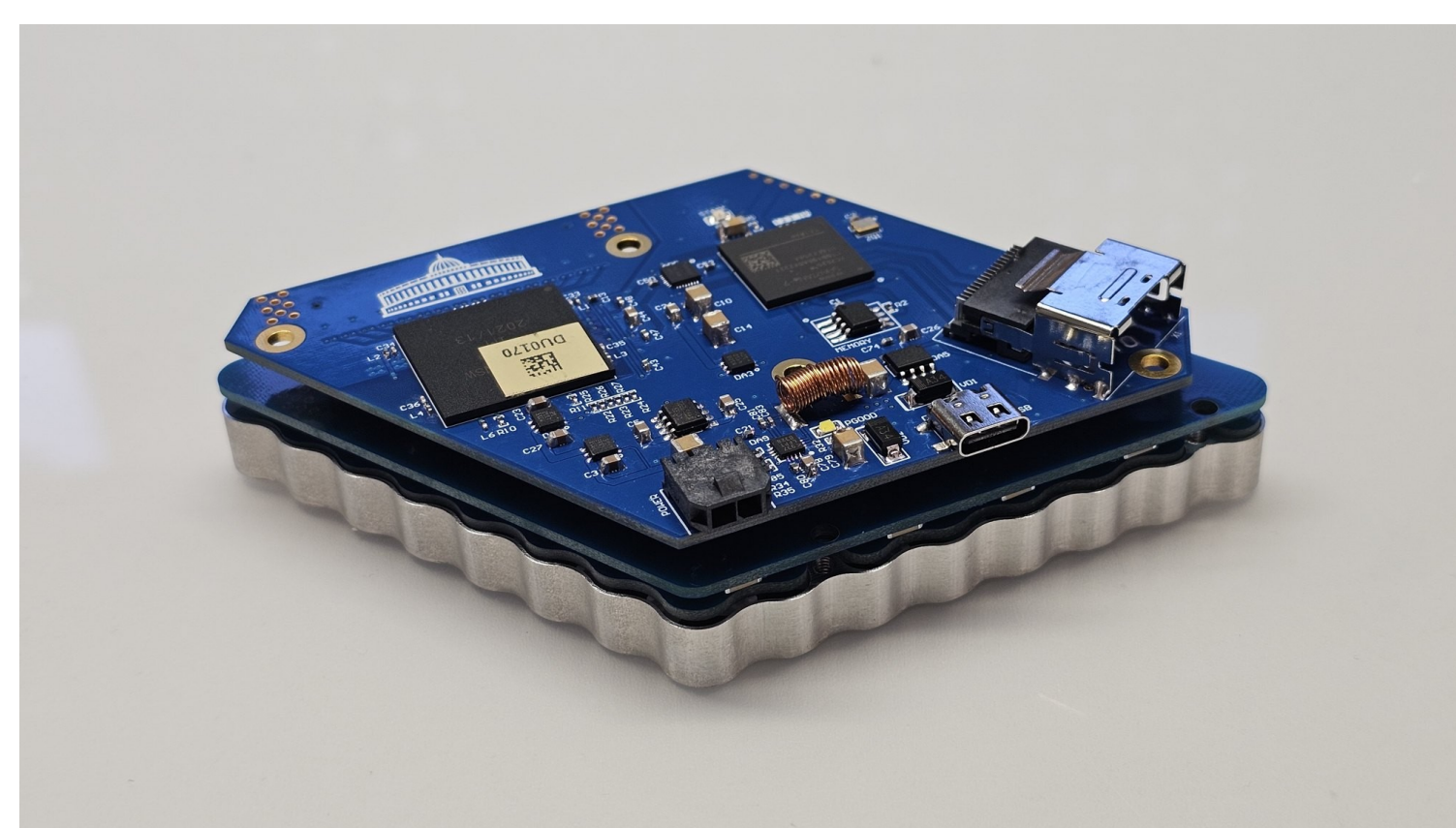
Readout “diamond” on the barrel high-voltage motherboard
