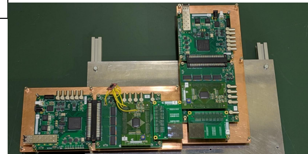
prototype MPPC readout with custom TF01A64 ASIC
