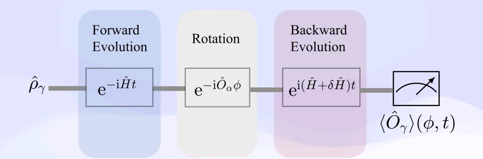
$$F(\phi, t) = Tr[\hat{O}_{\gamma}\hat{V}(t)e^{-i\hat{O}_{\alpha}(t)\phi}\hat{O}_{\gamma}e^{i\hat{O}_{\alpha}(t)\phi}\hat{V}(t)]$$
