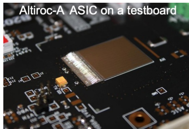
ASIC chip testing in test board
