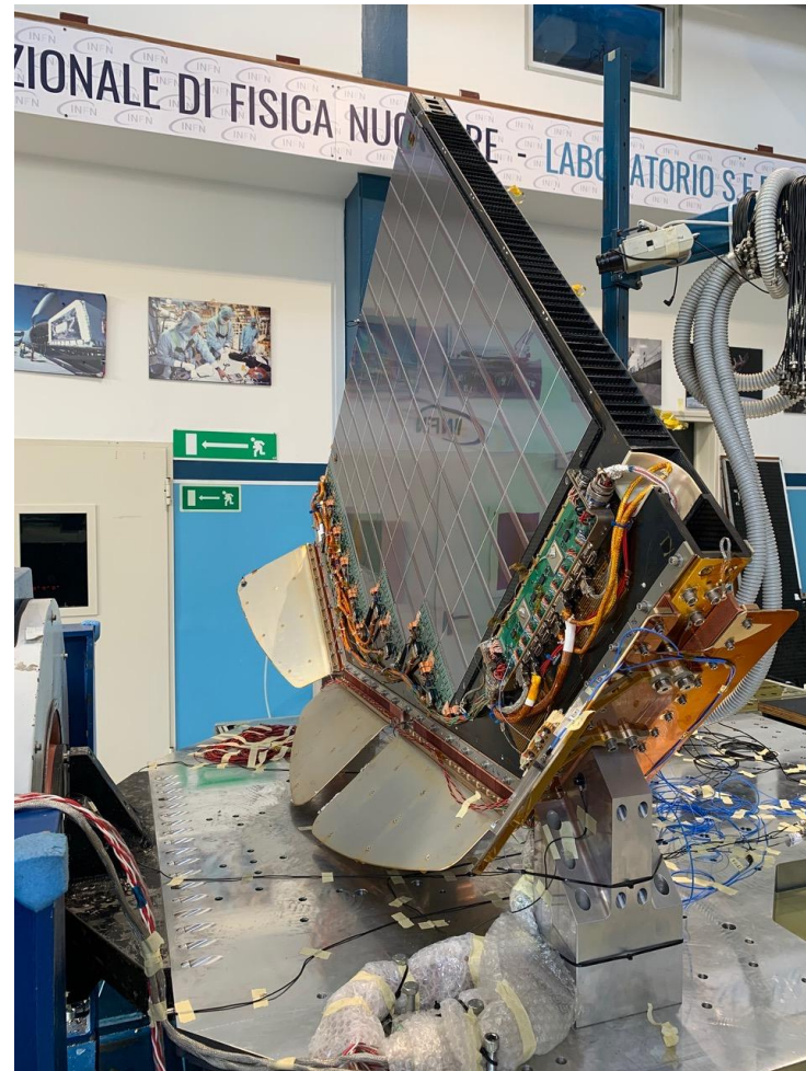
vibration test: no bonding-wire failure
