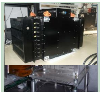
Sc-W ECAL: 30 layers, 1 \times 4.5 \text{ cm}^2 cells
