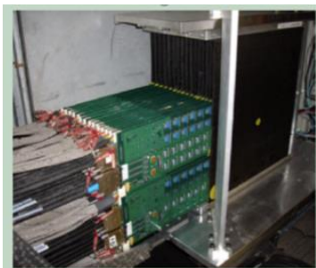
Si-W ECAL: 30 layers, 1 \times 1 \text{ cm}^2 cells
