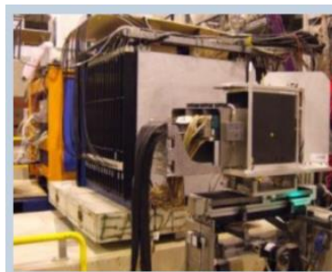
Sc-AHCAL, Fe&W: 38 layers, 3 \times 3 \text{ cm}^2 cells
