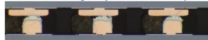
Wafer-to-wafer bonding of daisy-chain test wafers with Cu pillars
