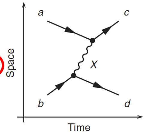
The Feynman diagram for the scattering process  $a + b \rightarrow c + d$  and the two time-ordered processes that it represents.
