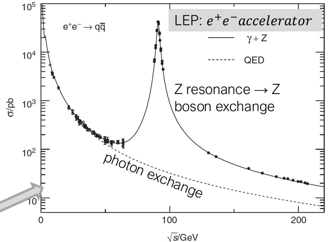
The measurements of the  $e^+e^- \rightarrow q\bar{q}$  cross section from LEP close to and above Z resonance. Also shown are the lower-energy measurements from earlier experiments. The dashed line shows the contribution to the cross section from the QED process alone. Adapted from [LEP and SLD Collaborations \(2006\)](#).
