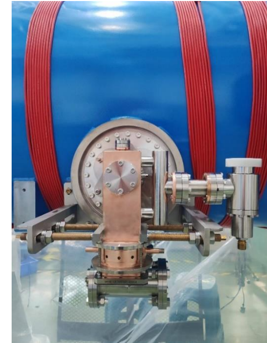
Fig. 3.9GHz FPC in cryomodule
