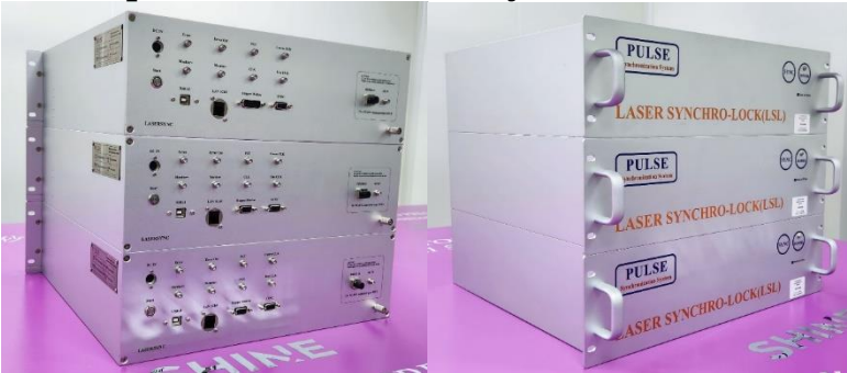
RF station synchro-controller
