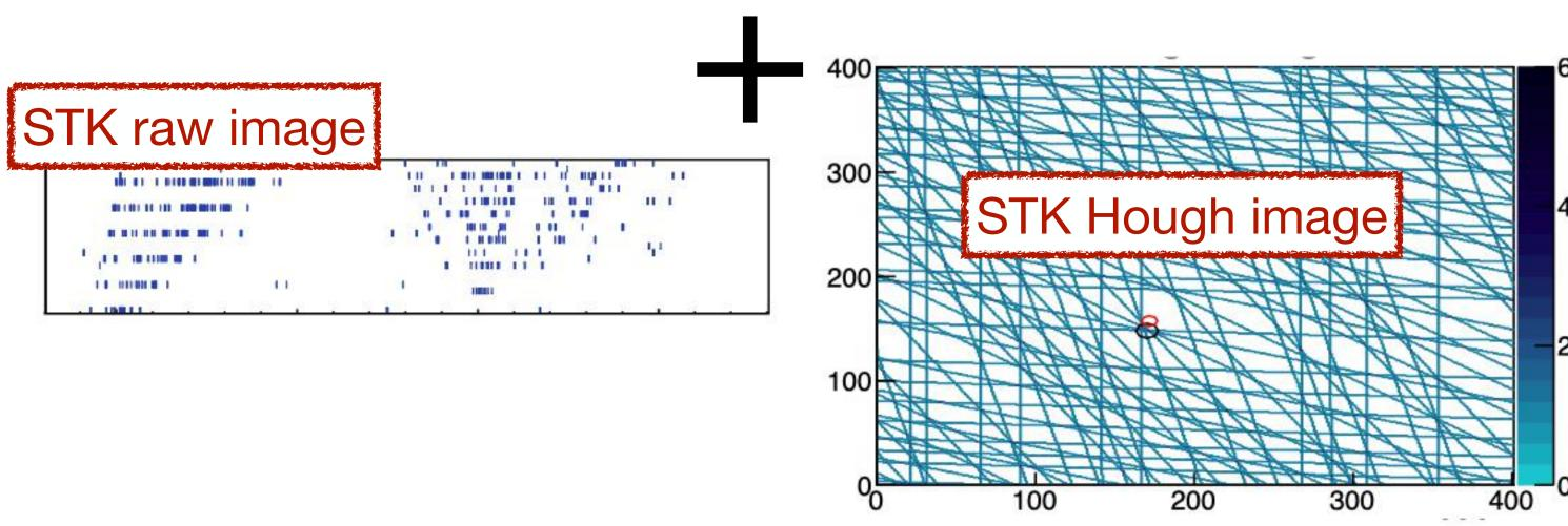
CALO & Tracker "images" used as input, regression type of problem — returns particle direction as an output (no track selection needed)
