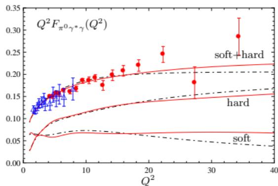
The “hard” and “soft” contributions to the  $\pi^0\gamma^*\gamma$  form factor for Model-I (solid curves) and Model-III (dash-dotted curves).
