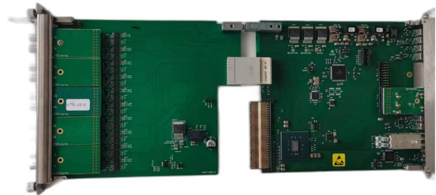
Figure The Rear-Transition Module for trigger distribution
