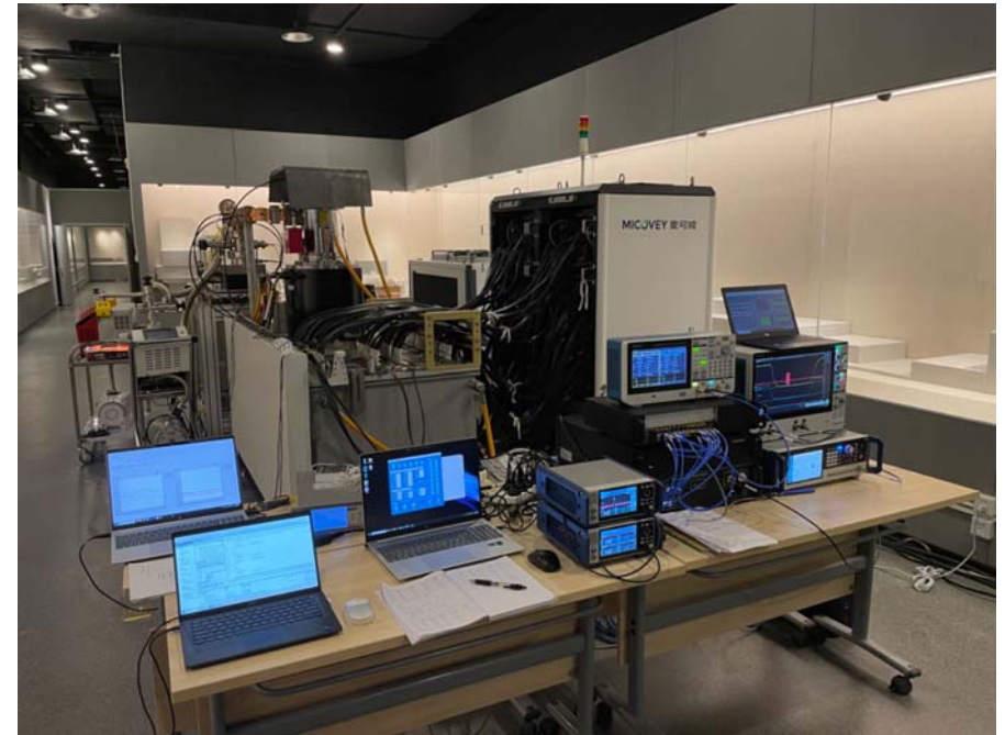
Testing and acceptance platform for klystron
