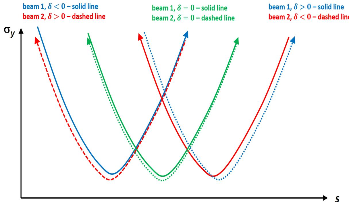
Waist location for beam 1 with momentum offset  $\delta$ , can be made to coincide with the waist location for beam 2 with momentum offset  $-\delta$ , leading to an effective monochromatization, without adding any new hardware.
