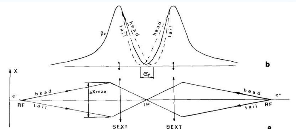
Fig. 6. a) The trajectories of the head and the tail of the bunch in the region between AS. b) The behaviour of  $\beta_z$ -function.
