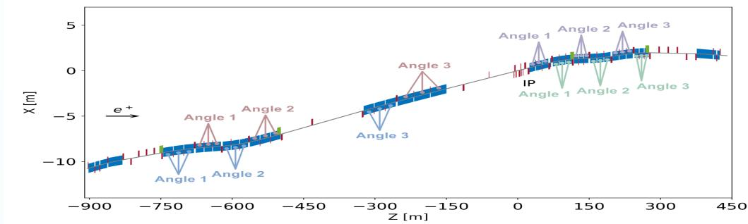
**Step 3:** The IP beam parameters are matched to FCC-ee MonochroM self-consistent parameters\* while keeping the beam parameters at the entrance and exit of the IR similar to those of standard mode, including phase advances between sextupoles and crab sextupoles.
