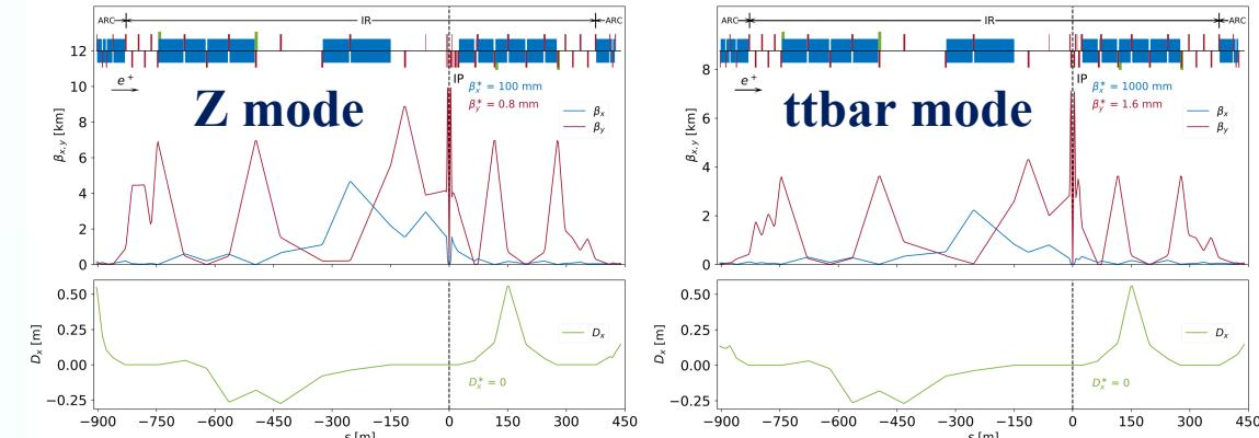
Highly asymmetric IR lattice around the IP to mitigate the SR impact
