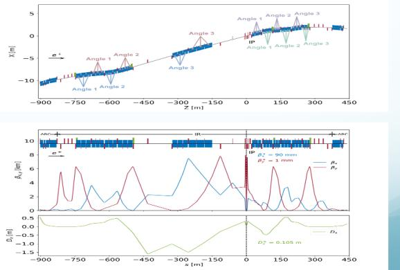
**Step 3:** The IP beam parameters are matched to FCC-ee MonochroM self-consistent parameters\* while keeping the beam parameters at the entrance and exit of the IR similar to those of standard mode, including phase advances between sextupoles and crab sextupoles.
