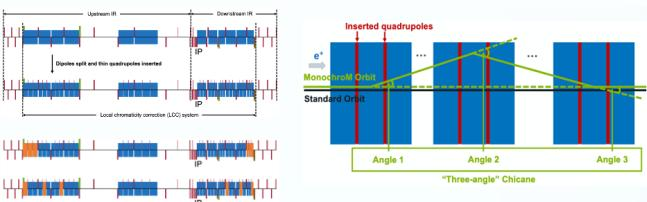
**Step 2:** To mitigate the horizontal emittance blowup, two long chicanes are implemented to each upstream and downstream. And each angle of chicane is equally distributed to all the three pieces of each LCCS H-dipole.
