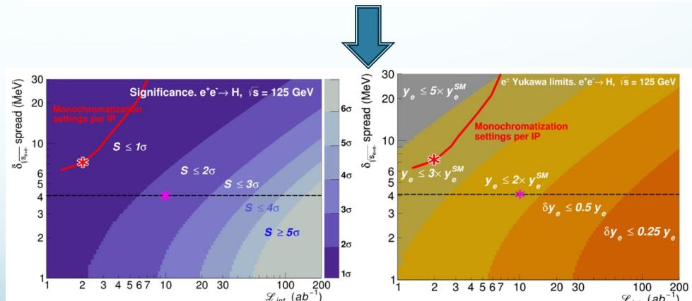
Significance contours in the  $\delta_{\sqrt{s}}$  vs.  $\mathcal{L}_{int}$  plane for  $\sigma_{ee \rightarrow H}$  cross section at  $\sqrt{s} = m_H$ .
