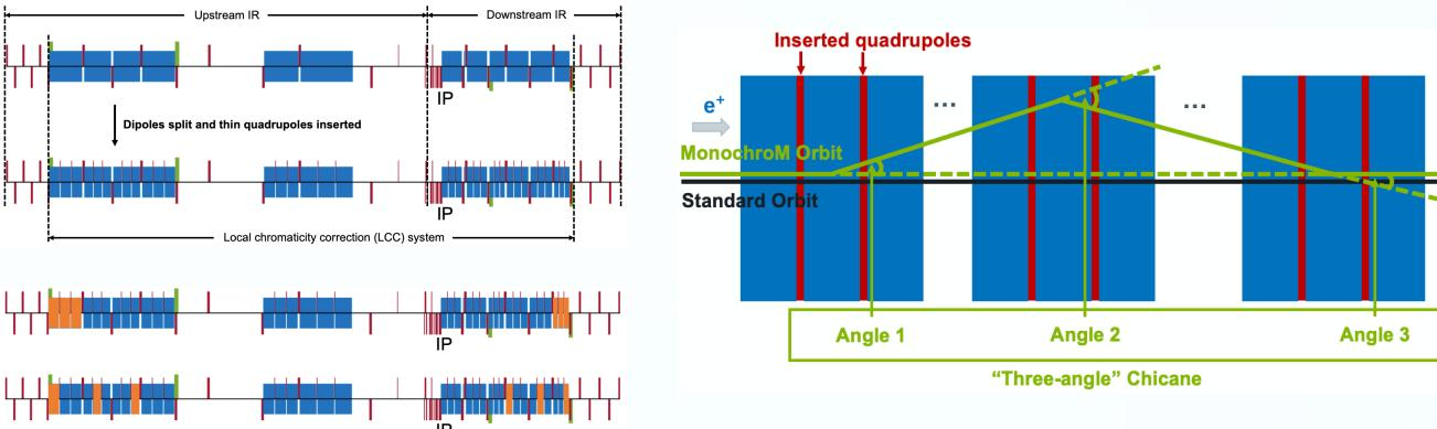
**Step 2:** To mitigate the horizontal emittance blowup, two long chicanes are implemented to each upstream and downstream. And each angle of chicane is equally distributed to all the three pieces of each LCCS H-dipole.
