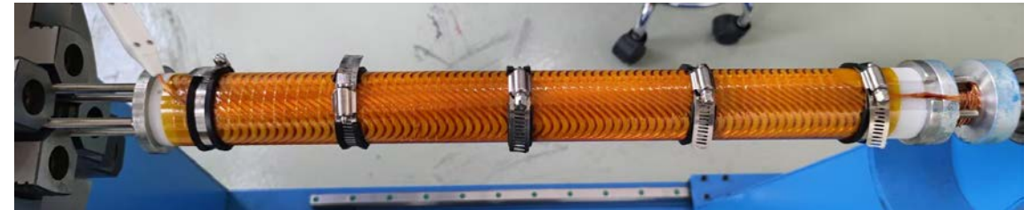
Trial winding on dummy former
