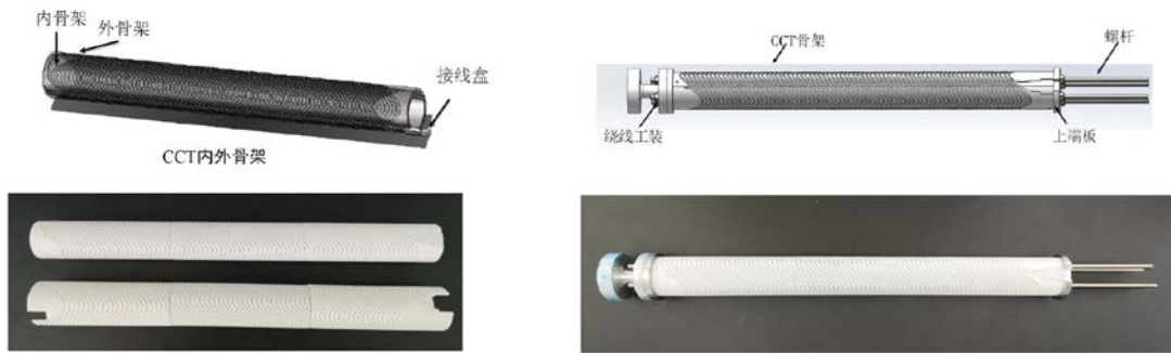
QD0 former drawing and 3D printing dummy former
