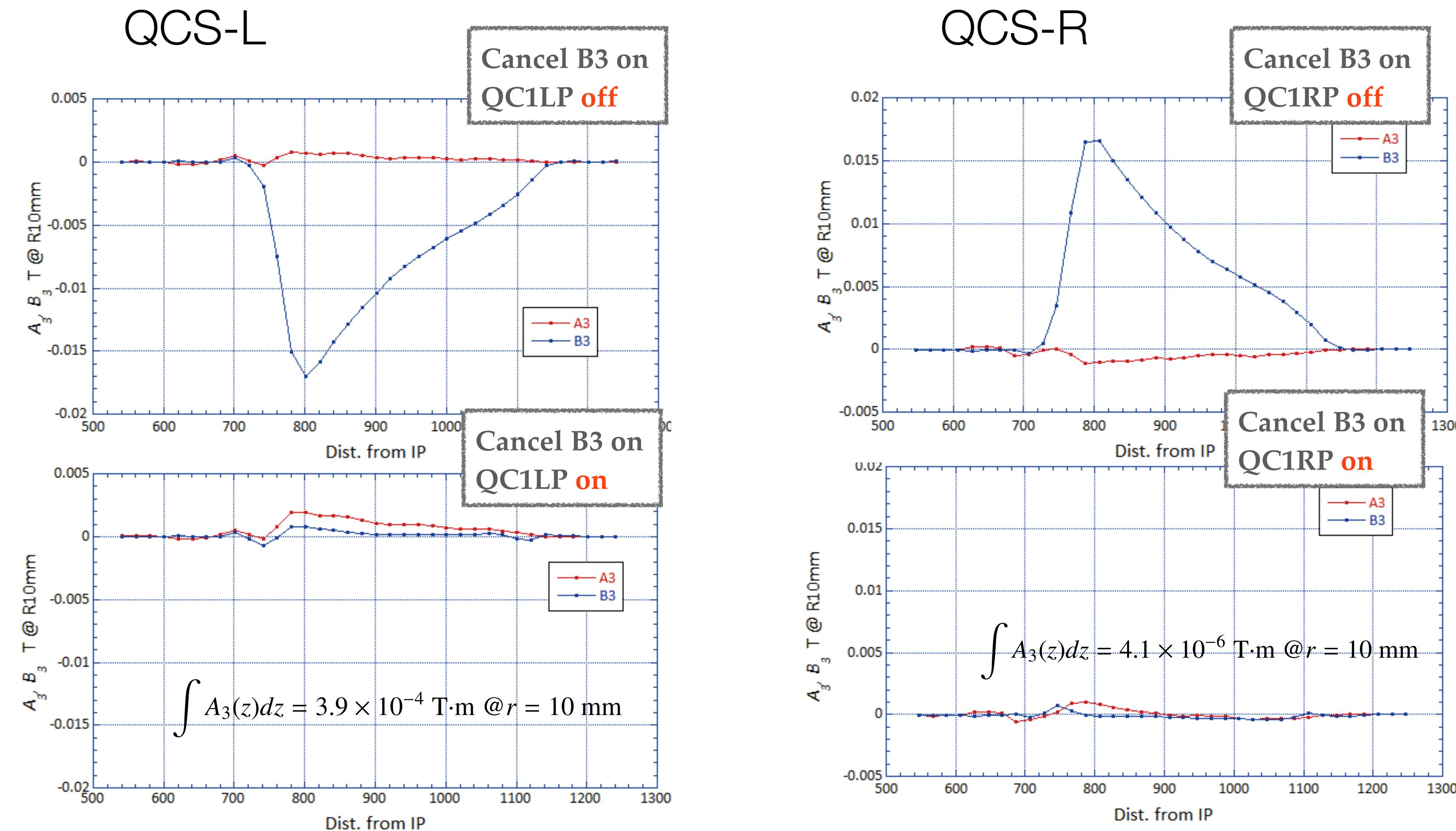
The energized current is optimized so that integral of  $B_3$  become to zero.
