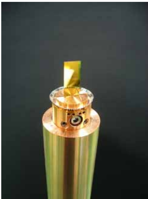
Diamond extraction mirror for visible light beam size monitor in holder
