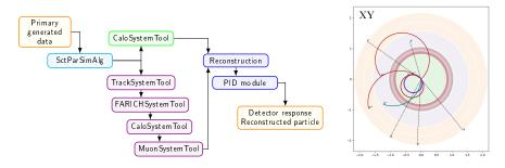
Takes primary particles from generator, produces result equivalent to reconstruction output (momentums, energies, PID)
