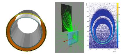
Takes primary particles from generator, G4 hits saved for later processing (digitization)
