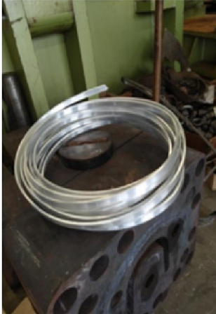
Al-stabilized NbTi/Cu superconductor
