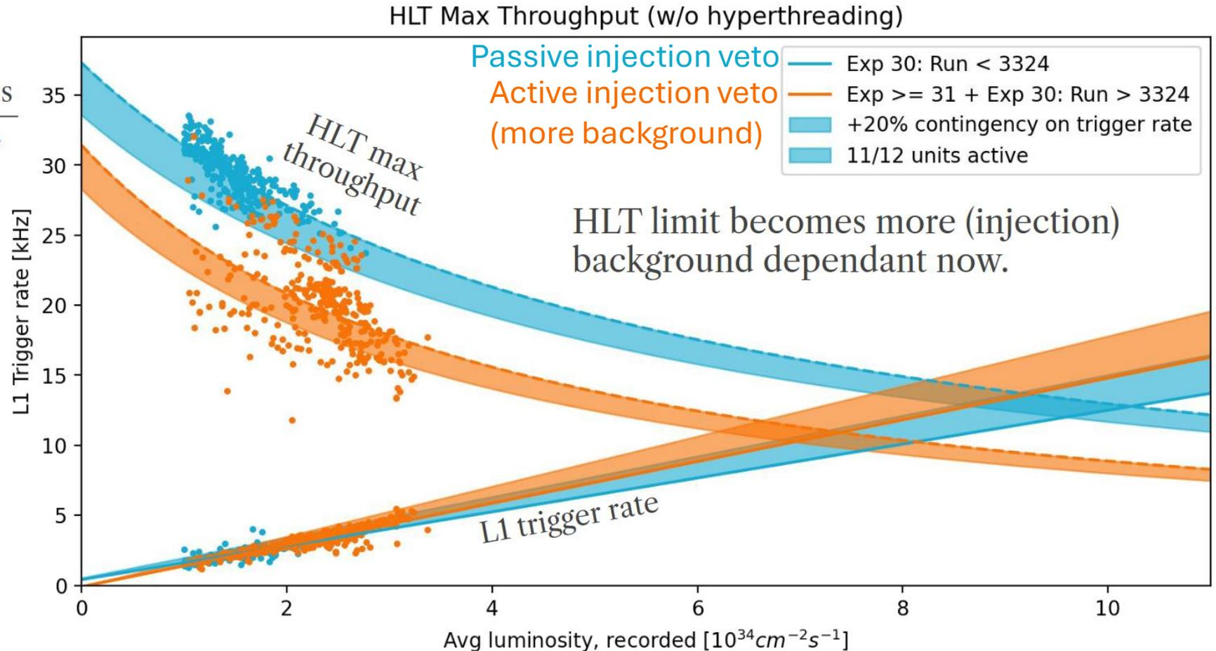
Based on early exp 30 → can operate up to  $9 \times 10^{34} / \text{cm}^2 / \text{s}$
