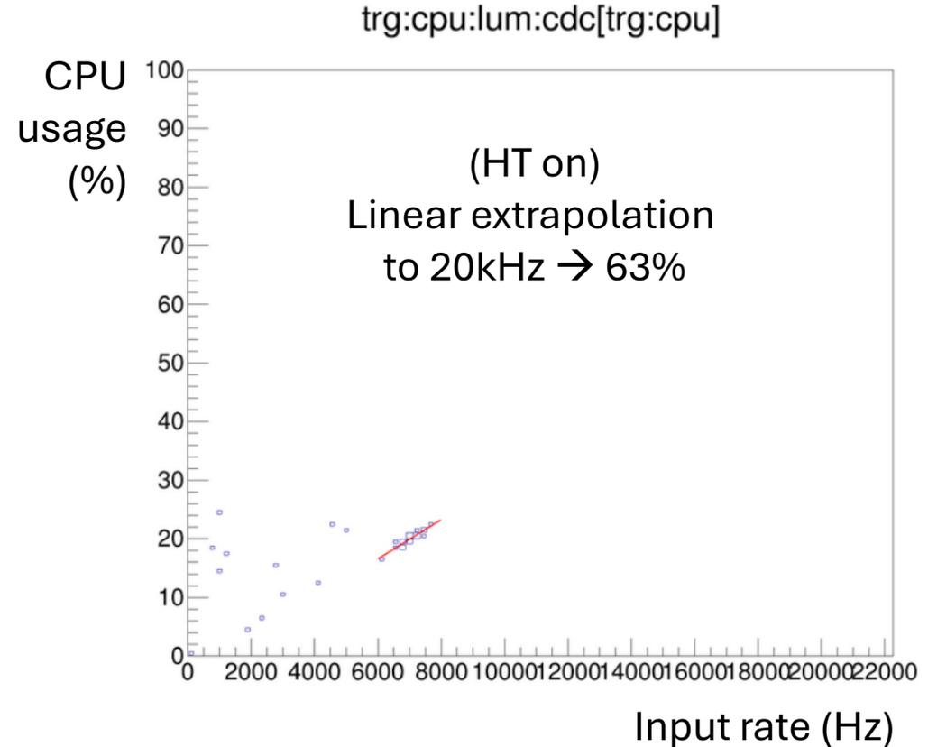
➤ Hyperthreading gives 1.5 times more computing power. By combining the result from the previous result, HLT (~6000-core) can handle 15-20 kHz
