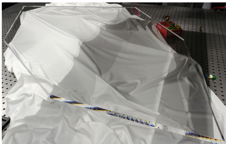
Full-size radiator plate from Nikon Corp, Japan 1nm surface roughness
