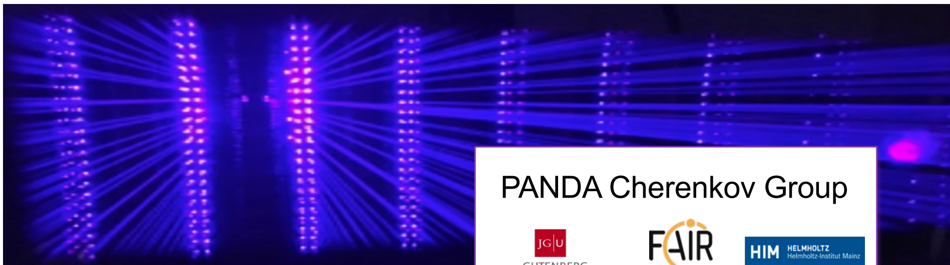
View into a DIRC bar with 442nm Laser light
