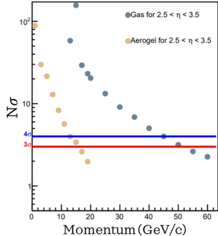
W/ **conservative 70% safety factor** [18 photo electrons](#) are detected. Over a wide range of rapidity required resolution is achieved. Region affected w/ spherical aberration are limited in momentum ( $6\sigma$  sep. upto **20 GeV/c**).
