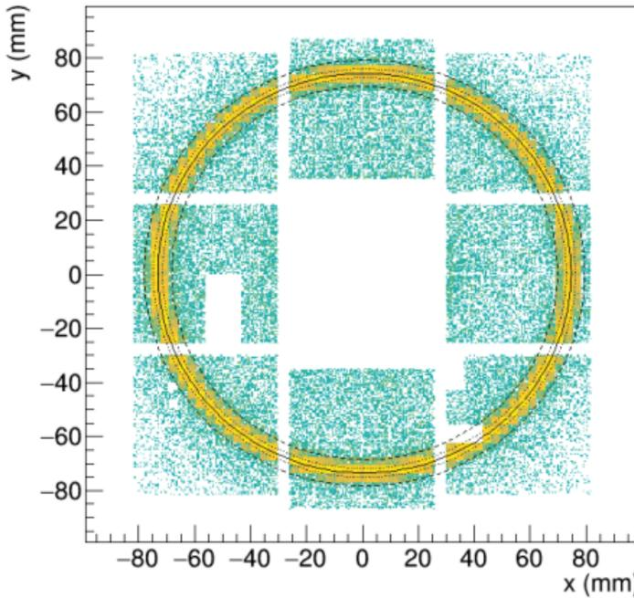
11.5 GeV/c negative beam, L = 4 cm n = 1.02 aerogel (accumulated events)
