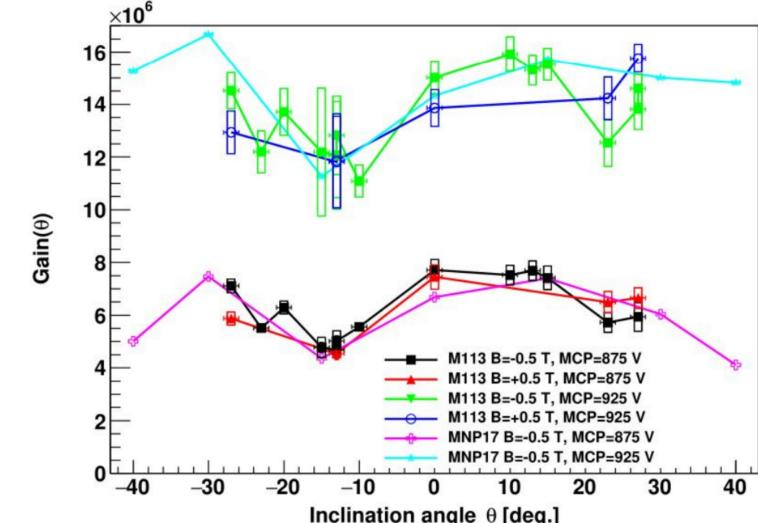
The overall performance of LAPPD in magnetic field is satisfactory. The drop in the gain and efficiency in high magnetic field values is observed. The drop is particularly present along the Chevron inclination and angle larger than 15 degrees. Most the loss can however be recovered by applying larger bias voltage across the MCP and increasing the photocathode voltage. The applied voltage can however vary from sensor to sensor
