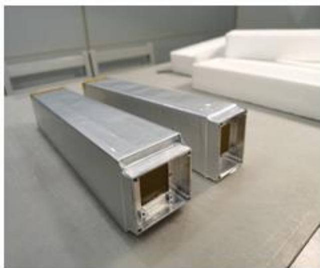
pCsl wrapped by Teflon & Mylar-Al film
