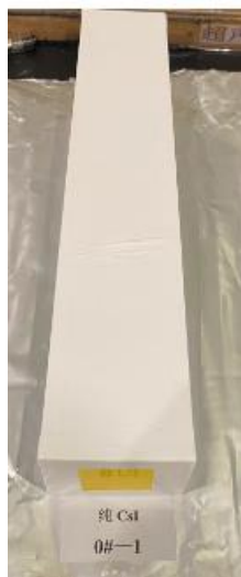
pCsl wrapped by Teflon & Mylar-Al film
