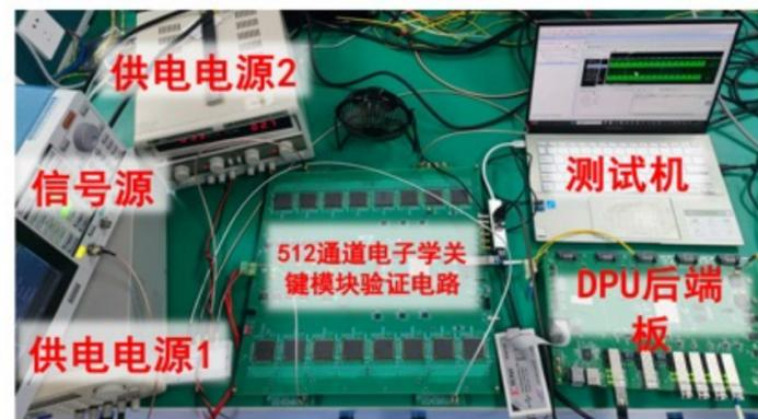
512-channel readout board using the self-developed ASIC
