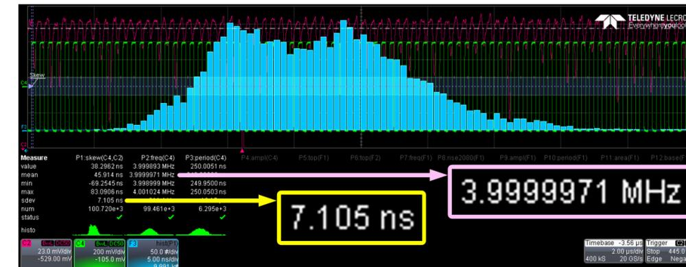
Tested the ASIC chip by feeding simulated detector output pulses to the chip at 4MHz with 35pF
