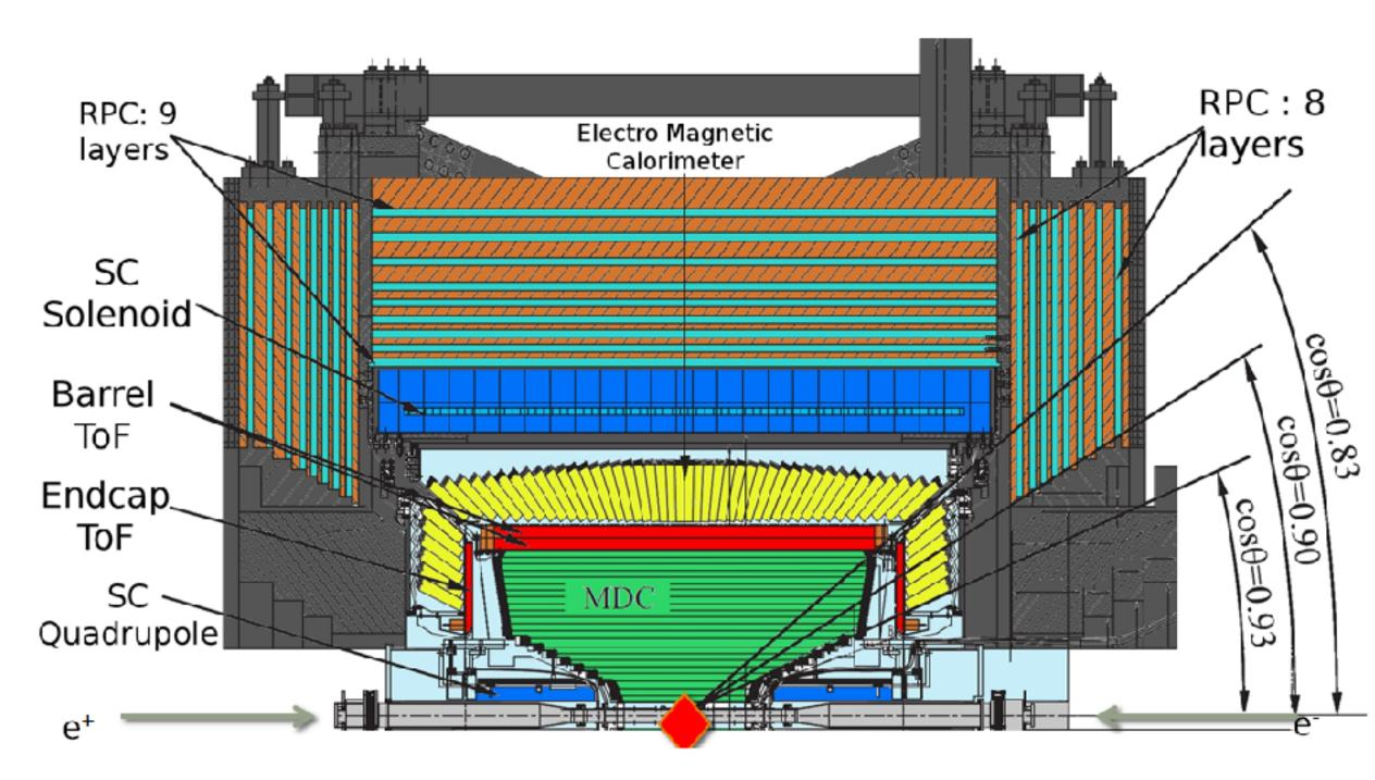
Total weight 730 ton, ~40,000 readout channel Data rate: 5kHz, 50Mb/s
