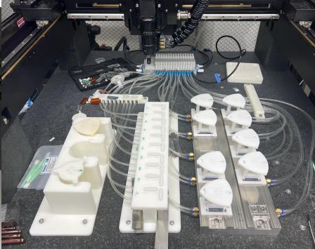
Picking tool   Picking dummy sensor   Placing dummy sensor
