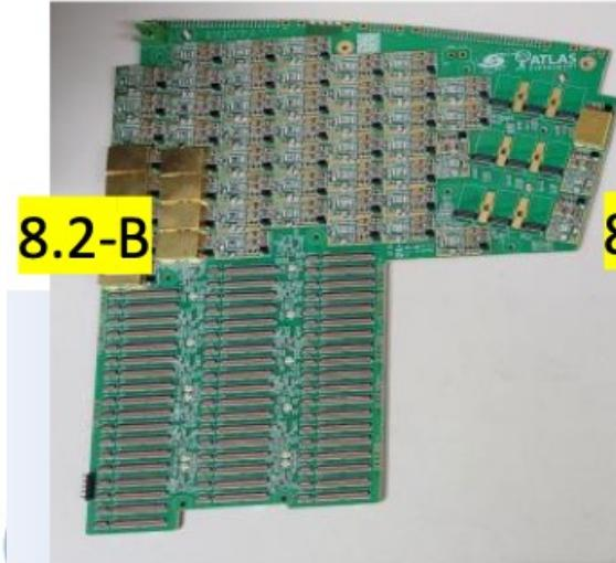
High voltage power supply prototype
