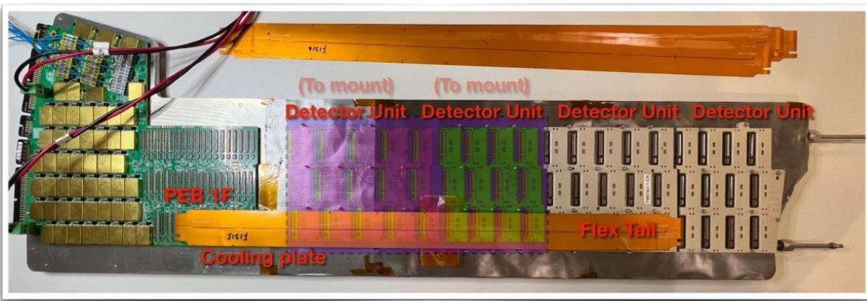
HV, LV, Cooling plate prototype
