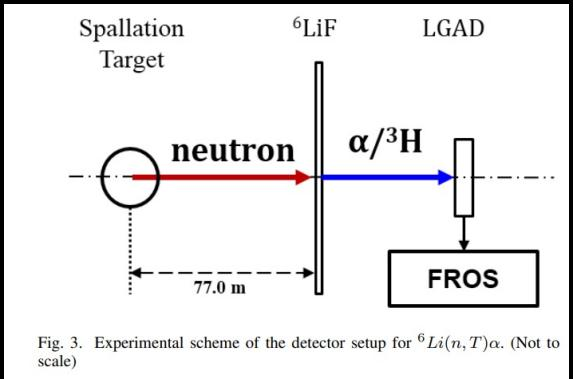
Fig. 3. Experimental scheme of the detector setup for  $^{6}\text{Li}(n, T)\alpha$ . (Not to scale)
