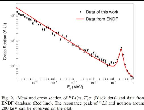
Fig. 9. Measured cross section of  $^{6}\text{Li}(n, T)\alpha$  (Black dots) and data from ENDF database (Red line). The resonance peak of  $^{6}\text{Li}$  and neutron around 200 keV can be observed on the plot.
