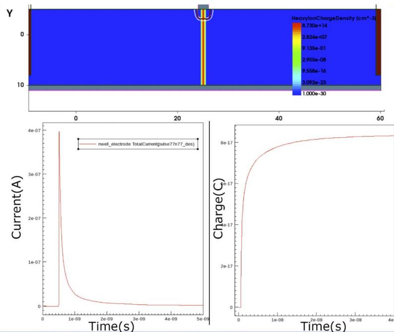
Charge collection situation for hit in the center of the diode
