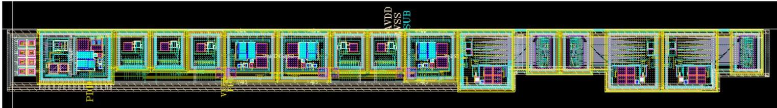
Bandgap, 8bit VDAC and 8bit IDAC
