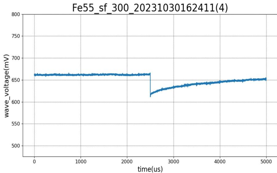
55 nm CIS工艺, Fe55源, 源跟随输出波形50mV
