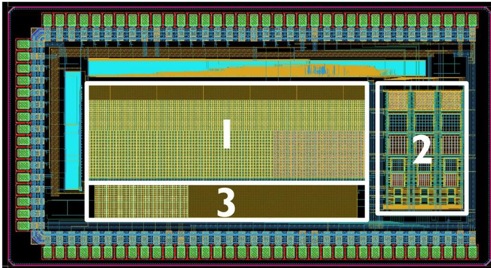
Figure: layout of the 1<sup>st</sup> prototype, consists of 3 big matrices for various purposes; including 3 pixel pitches ( $8\mu\text{m} \times 8\mu\text{m}$ ,  $16\mu\text{m} \times 16\mu\text{m}$  &  $24\mu\text{m} \times 24\mu\text{m}$ )
