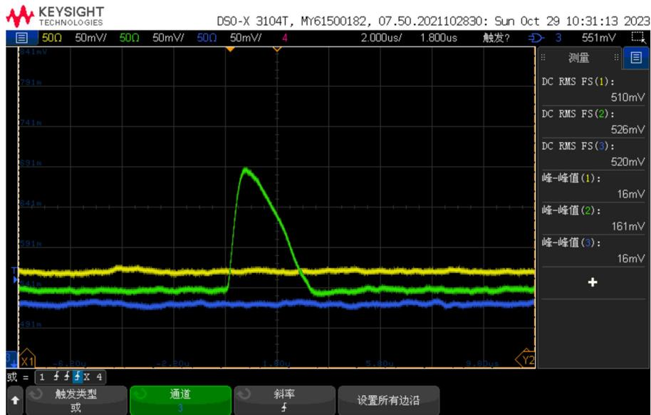
55 nm CIS, Fe55源, 模拟前端输出波形150mV
