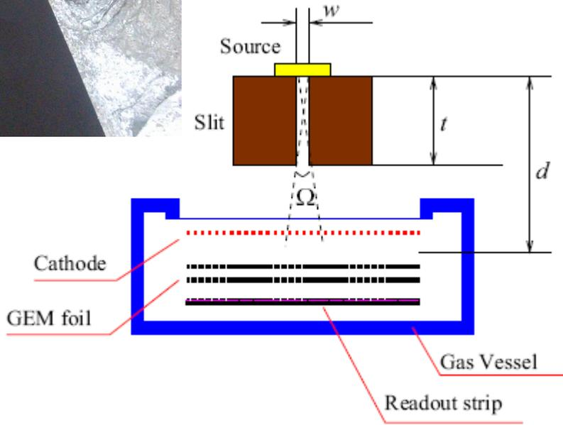
Schematic diagram of the slit system
