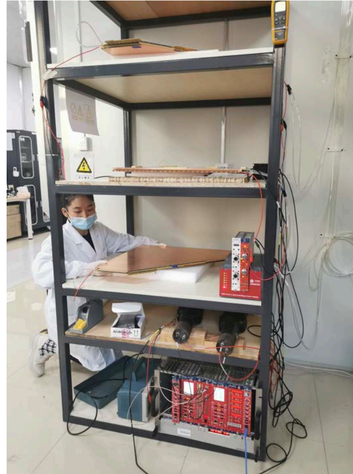
sTGC module test at SDU
