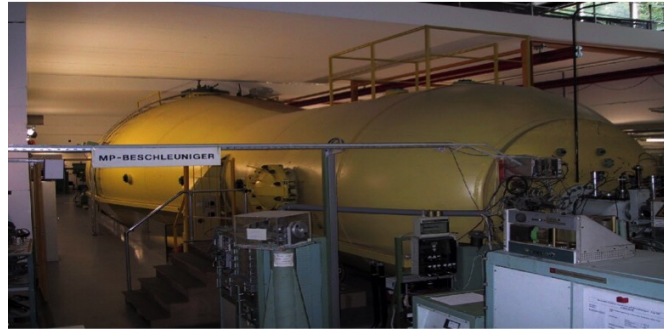
Fig. 6: A typical example of a tandem Van de Graaff accelerator; these are very reliable machines for precise measurements in atomic and nuclear physics. (Photo courtesy of the Max Planck Institute for Nuclear Physics, Heidelberg.)
